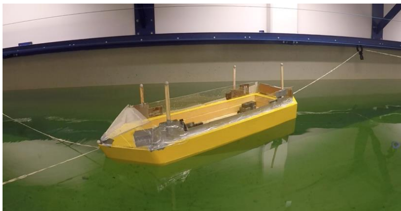
Figure 10: Light ship with ballast, loading condition LC1.
