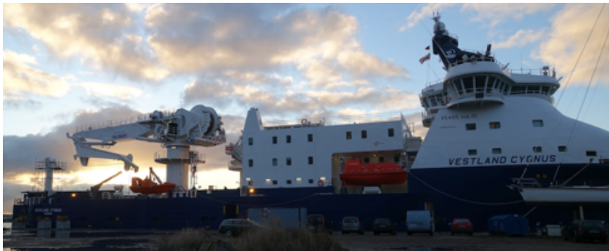
Figure 1. A ship installed with a stiff boom crane
