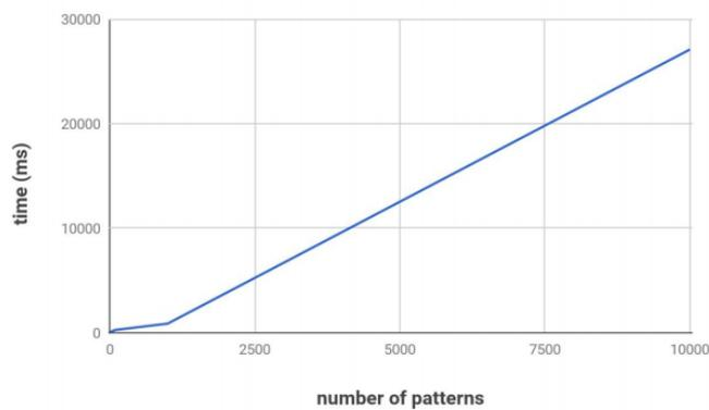
Fig. 5: Performance of the CEP System while increasing the no of stored patterns
