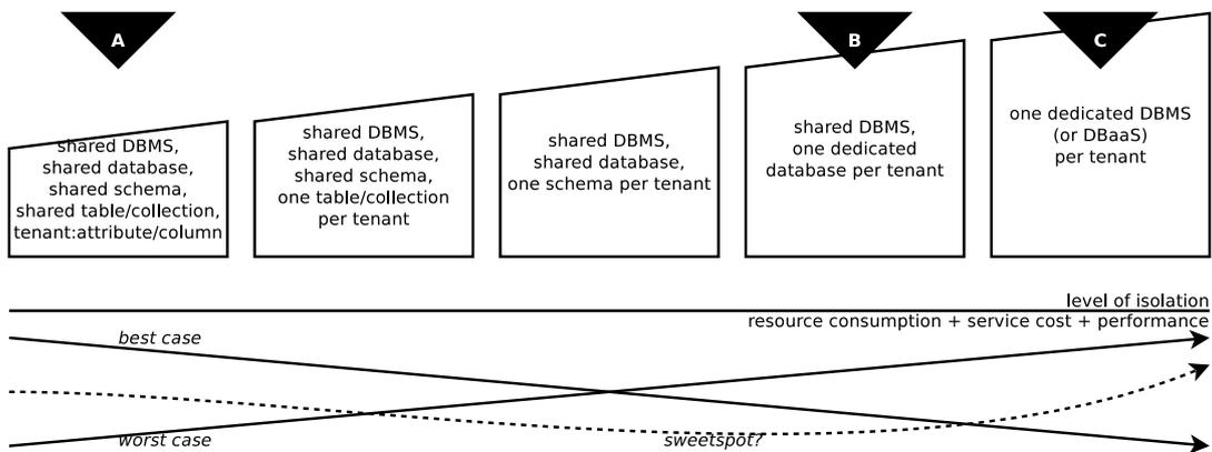
Fig. 9: Model of flexible multi-tenancy configurations for database services, with MongoDB
