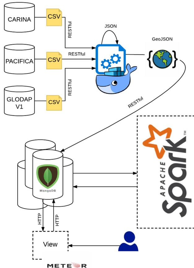
**Fig. 1.5.** The workflow includes the data acquisition and integration phases, considering the CSV format databases (CARINA; PACIFICA and GLODAP). A NoSQL solution stores all the GeoJSON information and integrates well with data analysis tool, such as Apache Spark, and MEAN stack web application, such as the Meteor JS framework. The dotted lines indicates guidelines for future works.
