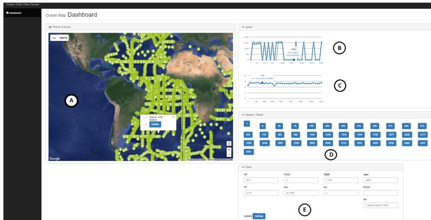
**Fig. 1.4.** Overview of the ODVServer platform. The layout was divided into two side. The first one (A) provided a geographical representation of the reading. Indeed, the right side (B, C, D, E) provided the insight view of the selected station.
