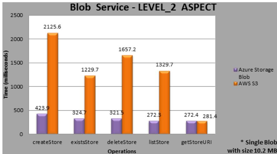
Fig. 3. Blob Service Level-2 Composite Object.
