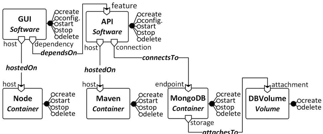
**Fig. 3.** An example of multi-component application specified in TOSCA (where nodes are typed with *tosker.nodes.Container*, *tosker.nodes.Volume*, or *tosker.nodes.Software*, while relationships are typed with TOSCA normative types [27]).
