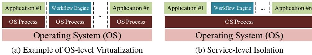
**Fig. 1** OS-level virtualization requires having separate OS processes for each tenant application and the workflow engine while service-level isolation allows running all code inside a single OS process.
