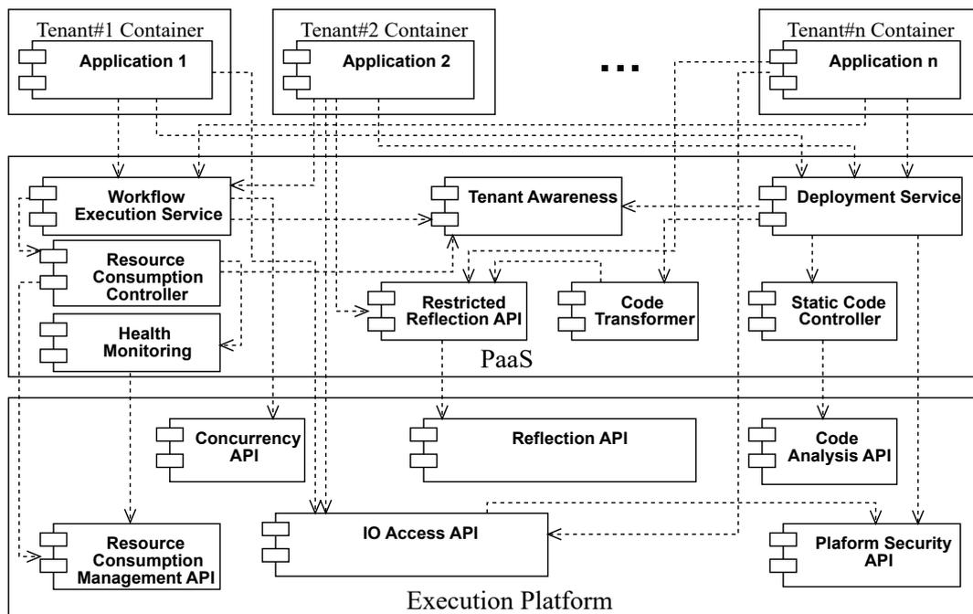
**Fig. 2** Building Blocks of the Framework in Relation to Tenant Applications and Execution Platform
