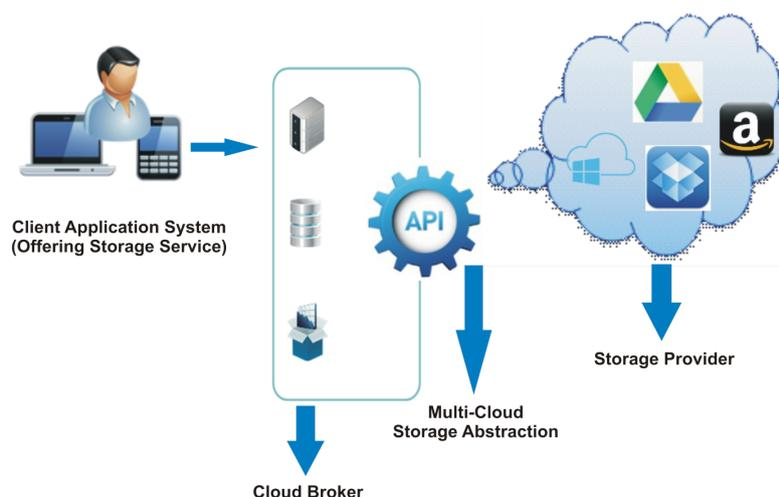
**Fig. 1.** Service brokerage architecture for cloud storage.
