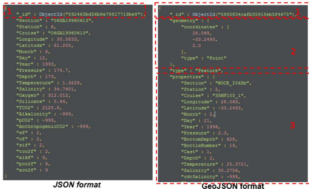
Fig. 1.6. Difference structure of JSON and GeoJSON
