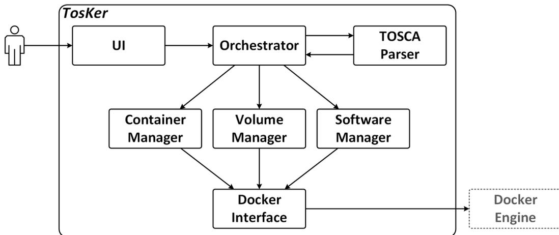
**Fig. 4.** The architecture of TOSKER.
