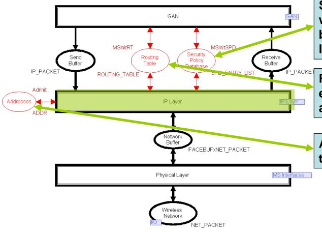
SPD: used by IPsec to specify which packets are allowed to be sent/received by the IP layer module
