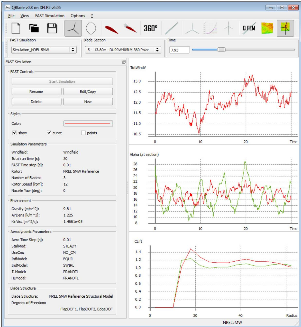
figure 16: The FAST Unsteady Aeroelastic Simulation module
