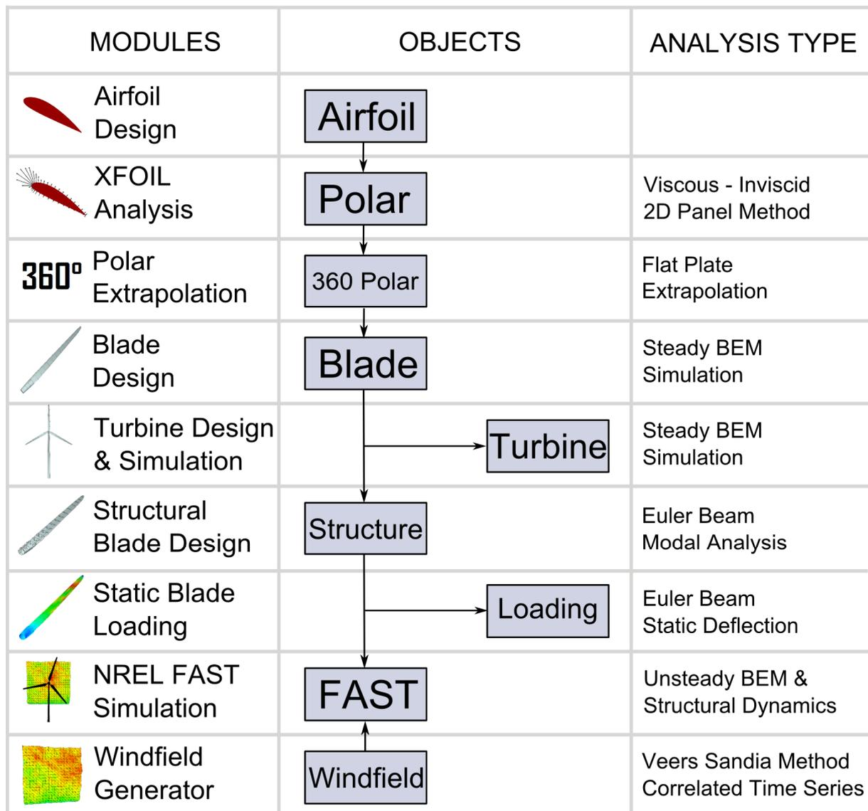
figure 2: QBlades object structure, modules and analysis types
