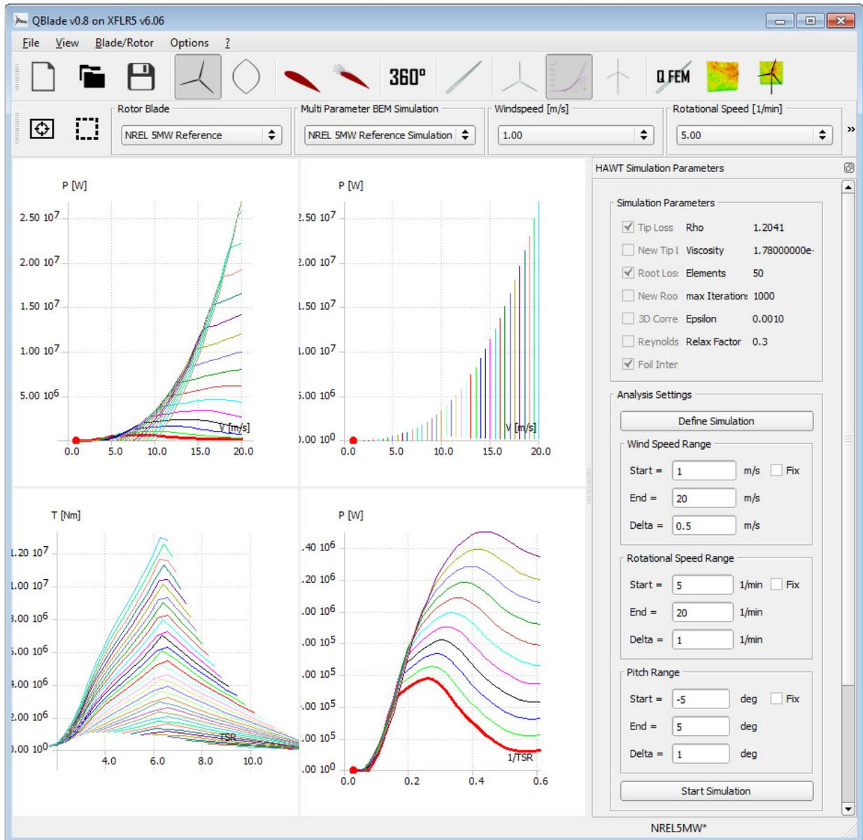
figure 11: The Multi Parameter Simulation module
