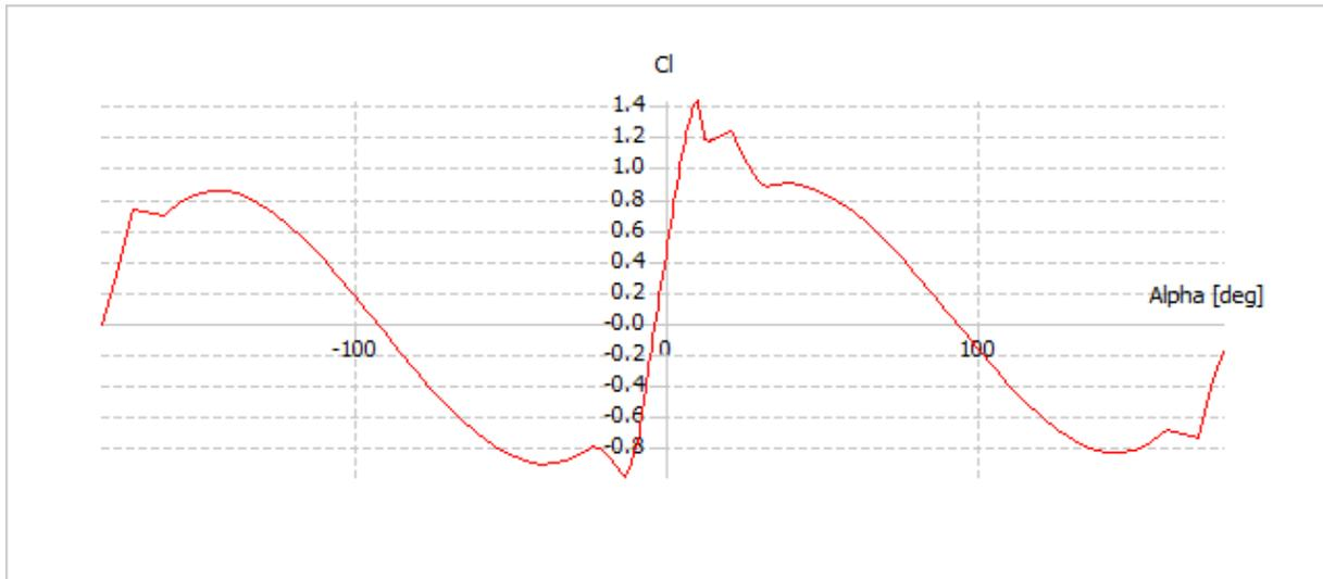
figure 4: A QBlade graph with a 360° polar curve object inside
