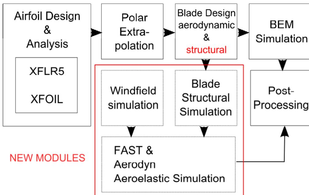
figure 1: Overview of the FAST coupling within QBlade
