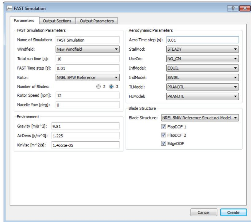
figure 17: Parameter tab of FAST Simulation dialog
