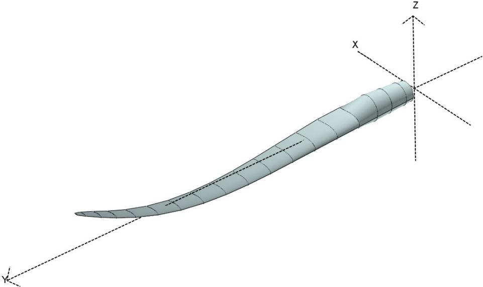
Flapwise Mode 2 Eigenfrequency: 4.56502 Hz
