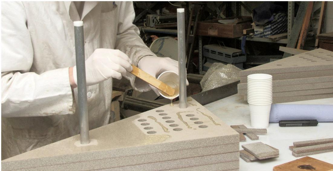
**Figure 2.2:** *Laminated construction of a buoyancy unit. The Divinycell profiles to be glued are on the right hand side of the picture. The two vertical alloy bars with white endings are structural braces used to attached the float to the other parts of the model. They also ensure that the profiles are well aligned with each others. The hole pattern is for ballasting (see figure 2.1).*
