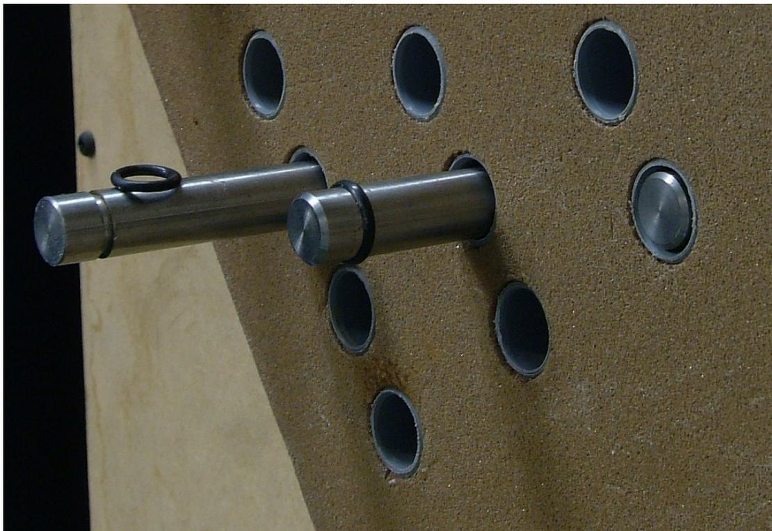
**Figure 2.1:** *Ballast weight arrangement in a Divinycell buoyancy unit. The holes are lined with grey PVC tubes. The left most bar is shown not fully inserted in the tube with the o-ring not fitted to show the groove. On the middle bar the o-ring is fitted and the right most bar is fully inserted in the tube.*
