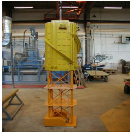
Figure 4.1 Scale model of a spar truss platform. Source from Montasir and Kurian (2011). The horizontal plates attached to the truss are employed to decrease the vertical motions of the structure.
