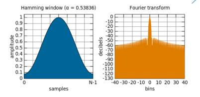
The signal is segmented into «windows». The FFT is computed segment by segment which are then assembled to give the PSD.
