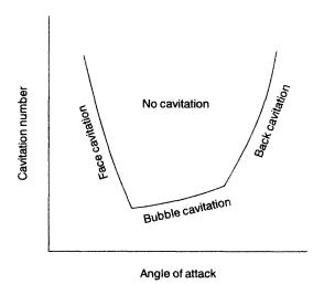
Figure 9.17 Cavitation bucket
