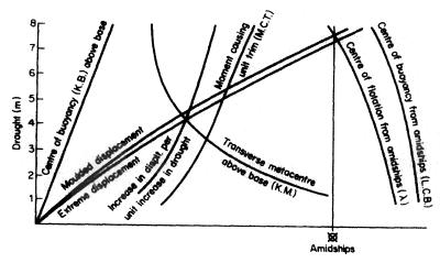
Figure 4.11 Hydrostatic curves
