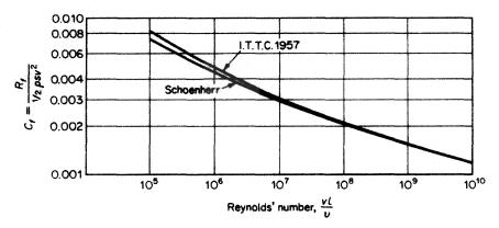
Figure 8.8 Comparison of Schoenherr and ITTC 1957 lines
