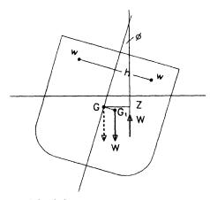
Figure 4.28 Transverse weight shift
