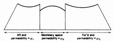
Figure 4.38 Floodable length with permeability
