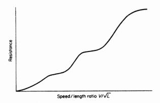
Figure 8.4 Humps and hollows in resistance curve
