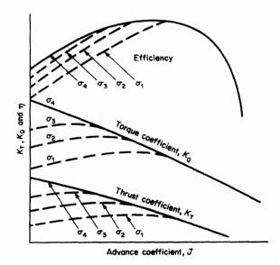
Figure 9.19 Propeller curves with cavitation
