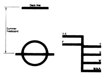
Figure 2.5 Load line markings
