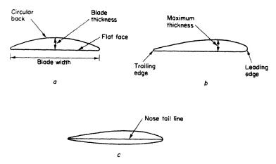
Figure 9.5 (a) Flat face, circular back; (b) Aerofoil; (c) Cambered face
