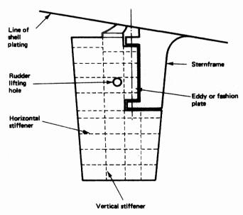
Figure 10.7 Semi-balanced rudder
