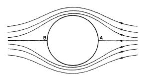
Figure 9.8 Flow round circular cylinder
