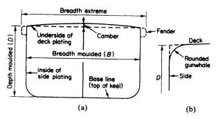
Figure 2.2 Breadth measurements
