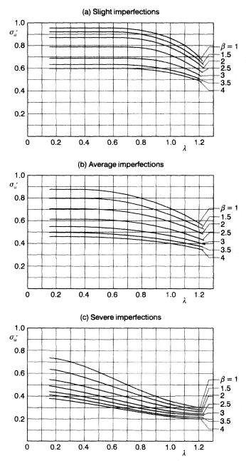
Figure 7.17 Compressive strength of panels (courtesy RINA<sup>14</sup>)
