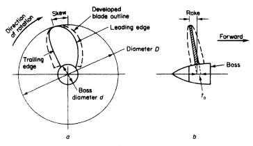
Figure 9.4 (a) View along shaft axis, (b) Side elevation
