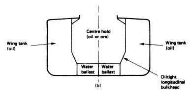
Figure 12.6 Section of oil/ore carrier
