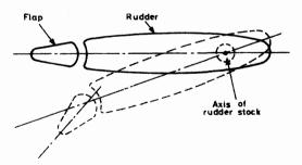
Figure 10.8 Flap rudder
