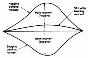
Figure 7.5 Still water and wave bending moments
