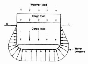
Figure 7.1 Loads on ship section
