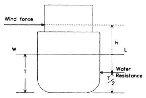
Figure 4.31 Heeling due to wind
