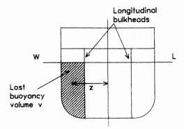
Figure 4.35 Asymmetrical flooding
