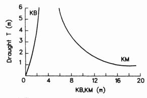
Figure 4.9 Metacentric diagram
