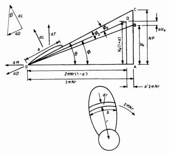
Figure 9.12 Forces on blade element
