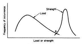
Figure 7.23 Load and strength distributions
