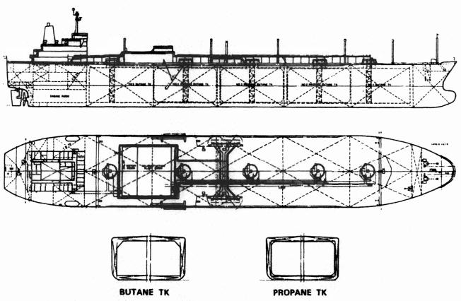
Figure 12.8 Liquefied petroleum gas carrier
