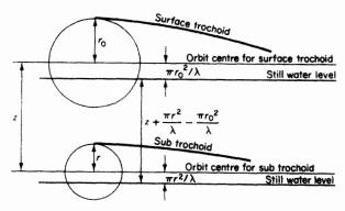
Figure 5.3 Pressure in wave
