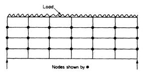
Figure 7.20 Beam finite elements
