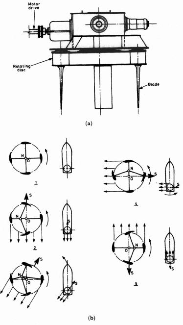
Figure 10.10 Vertical axis rudder (a) Construction (b) Operation
