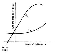
Figure 9.7 Lift and drag curves
