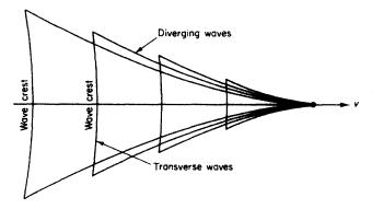
Figure 8.2 Pressure point wave system
