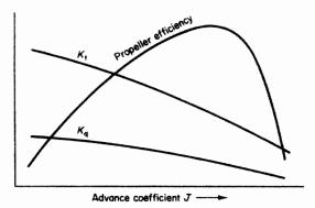
Figure 9.13 Thrust, torque and efficiency curves
