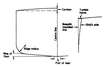
Figure 2.3 Section measurements
