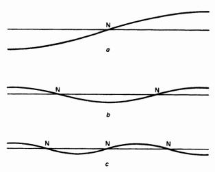
Figure 11.4 (a) One-node; (b) Two-node; (c) Three-node
