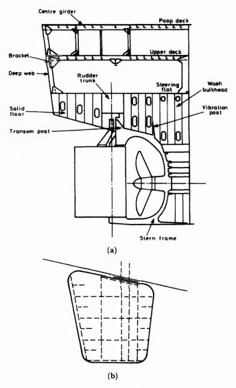
Figure 10.5 Balanced rudders (a) Simplex; (b) Spade
