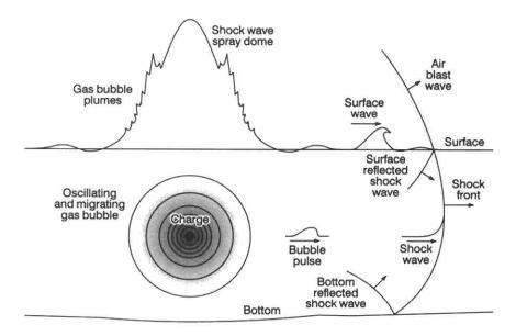
Figure 11.8 Underwater explosion (courtesy RINA<sup>18</sup>)
