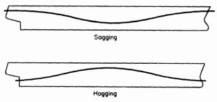
Figure 7.2 Ship on wave
