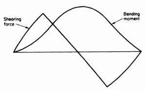
Figure 7.4 Shearing force and bending moment
