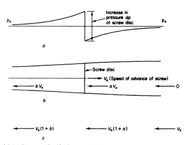
Figure 9.1 (a) Pressure; (b) Absolute velocity; (c) Velocity of water relative to screw
