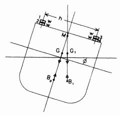
Figure 4.18 Inclining experiment
