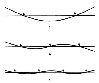
Figure 11.3 (a) Two-node; (b) Three-node; (c) Four-node
