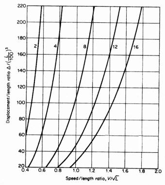
Figure 8.10 Contours of frictional resistance in pounds per ton displacement for  $500\,\mathrm{ft}$  ship
