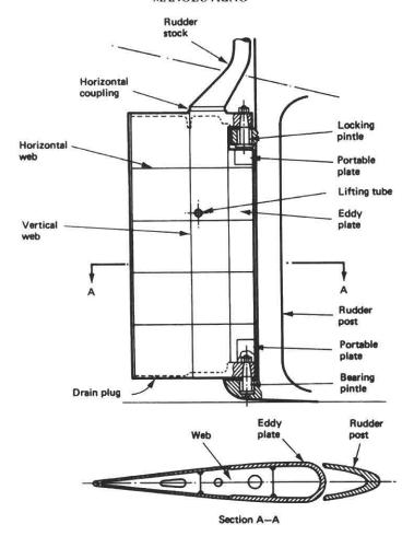
Figure 10.6 Unbalanced rudder
