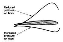
Figure 9.11 Pressure distribution on aerofoil
