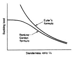
Figure 7.15 Comparison of strut formulae
