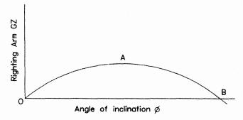
Figure 4.23 Curve of statical stability
