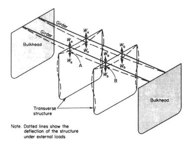
Figure 7.19 Transverse strains
