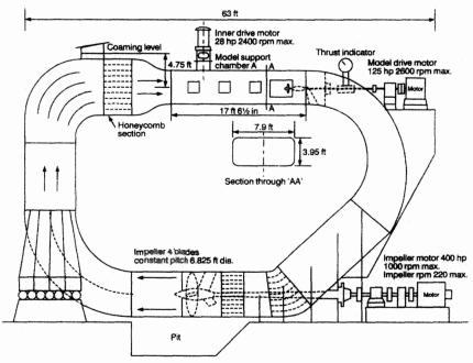
Figure 9.18 Large cavitation tunnel (courtesy RINA)
