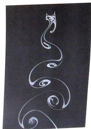
Figure 3.6 The Kármán vortex street in the wake of a cylinder.
