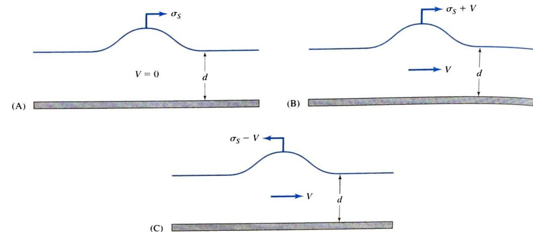
**Figure 3.5** Infinitesimal wave moves (A) to the right on stationary fluid (B) to the right on fluid moving to the right and (C) to the left on fluid moving to the right. To an observer moving with the fluid, the wave speed is  $\sigma_S$  in both cases. For an observer on the shore, the wave speed is  $\sigma_S$  for (A),  $\sigma_S + V$  for (B), and  $\sigma_S - V$  for (C).
