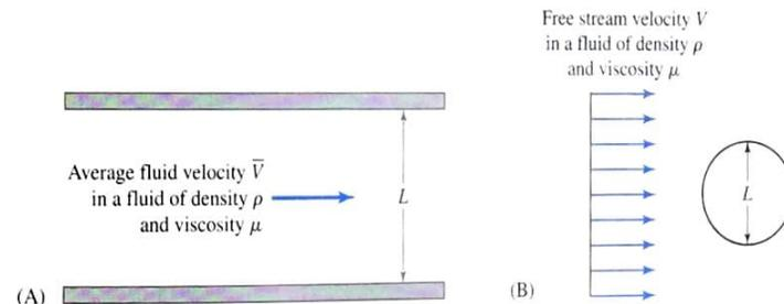
**Figure 3.2** Velocity and length scales used in defining  $Re$  for examples of (A) internal flow and (B) external flow.
