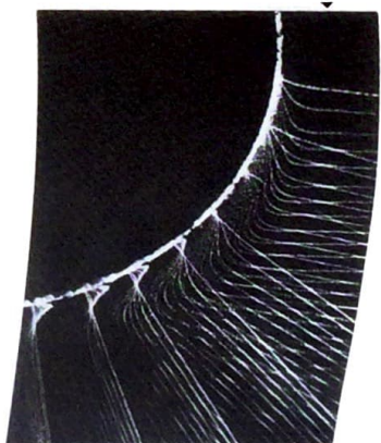
Figure 14.19 Flow visualization of the boundary layer on a cylinder created with hydrogen bubbles.
