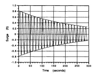
**FIGURE 10.16 EXTINCTION TEST OF A TANKER IN SURGE**
