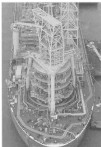
Figure 7.29 Internal bow turret (SBM-Imodco)
