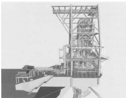
Figure 7.30 Cantilevered bow turret (SBM-Imodco)
