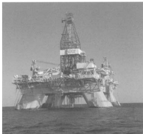
Figure 7.35 “Deepwater Nautilus” – 5th generation drilling semi-submersible (Photo courtesy Transocean)
