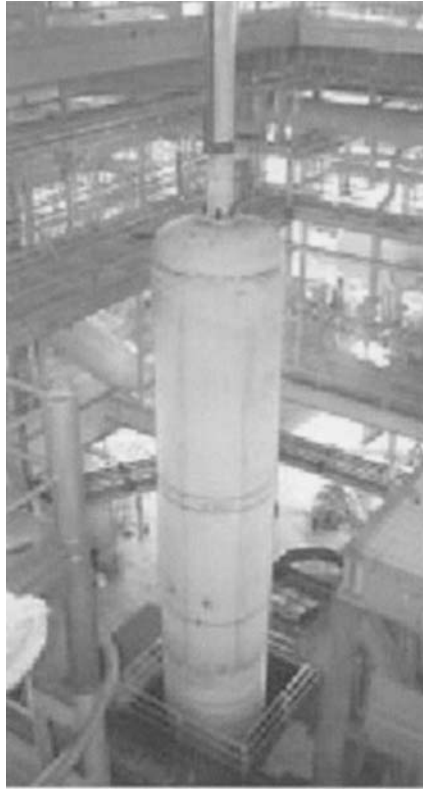
Figure 7.67 Buoyancy can being installed (Technip Offshore)
