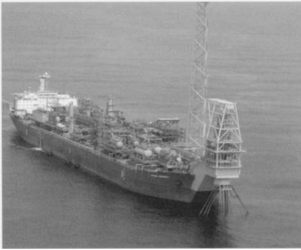
Figure 7.24 Xikomba with Bow Turret (SBM)
