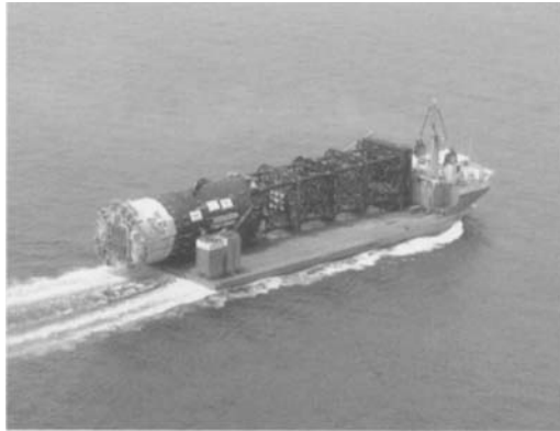
Figure 7.82 Transportation of the spar (Technip Offshore)
