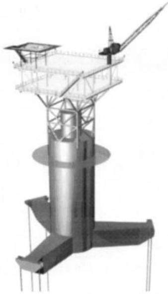
Figure 1.20 SeaStar Mini TLP (Courtesy Atlantia Corp.)
