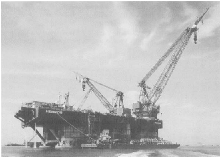
Figure 7.136 Semi-submersible crane vessel (Heerema Offshore)
