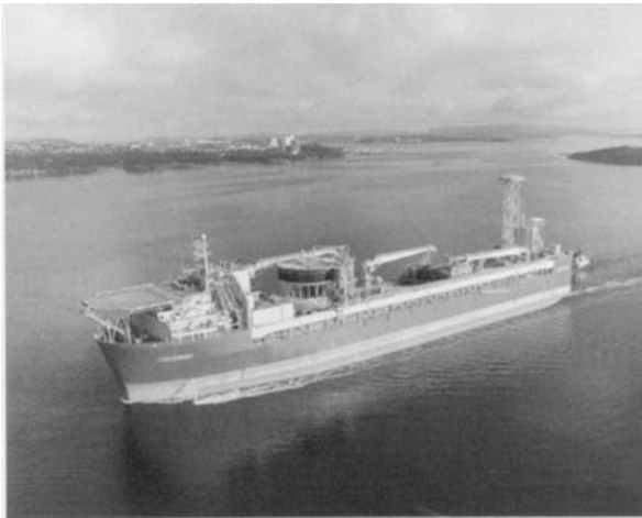
Figure 7.25 Balder FPSO with Turret Midships (ExxonMobil)
