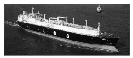
The 'DISHA', an LNG vessel. LBP = 266.0 m. LNG =  $138\,000\,\text{m}^3$ . Dwt =  $70\,150\,\text{t}$ . 17 Officers plus 21 crew.
