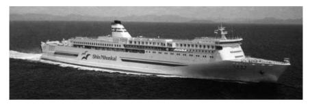
The 'HAMANASU', a Ro-Ro vessel LBP = 208.0 m. Dwt = 5824 t. Vehicles: 158 trailers/65 cars.
