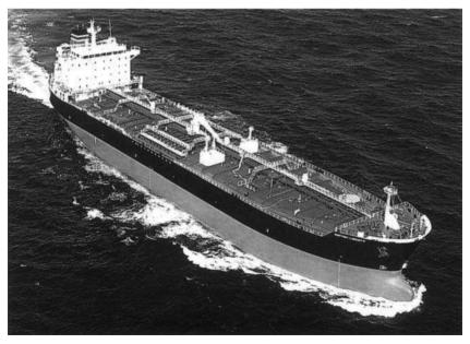
The 'BRITISH LIBERTY', a chemical carrier. LBP = 174.0 m. Dwt = 40 580 t. Built to class 1A ICE strengthening requirements.
