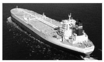
The 'HELLESPONT ALHAMBRA', an ULCC. LBP = 366.0 m. Dwt = 407 469 t. Double hull. Fuel consumption = 140.3 tonnes/day.
