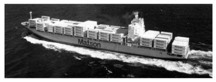
The 'MANUKAI', Container ship.  $LBP = 202.24 \, m. \, Dwt = 30\,000 \, t.$ Containers:Total TEU capacity = 3000.
